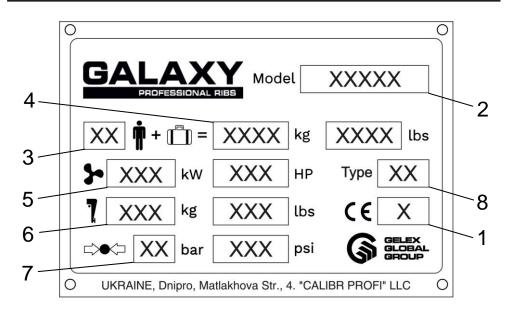
The indications on the capacity plate give information about limitations imposed by international regulations. Your local regulations can be different. Also these indications are not a complete list: the security requirements (obligatory security equipment of the boat, maximum authorized distance you can navigate from a shelter, etc.) may change according to the country or state.
