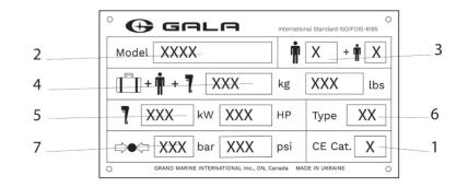
The indications on the capacity plate give information about limitations imposed by international regulations. Your local regulations can be different. Also these indications are not a complete list: the security requirements (obligatory security equipment of the boat, maximum authorized distance you can navigate from a shelter, etc. ) may change according to the country or state. Always refer to local regulations to be informed on actuall requirements.
