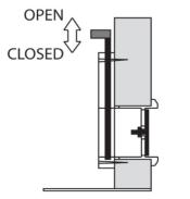
Overpressure valve protects the boat against unexpected pressure increase over the maximum working limit. In case of any tube pressure increase or overinflating the gasket of the valve will open automatically, release all excessive air and bring the tube pressure to nominal. Make sure that the valve cup is always clean. Check the valve operation during boat maintenance.
