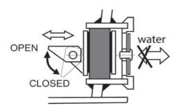
Drain valve includes: a) expanding plug inside of the cockpit with opening-closing lever, b) one-way drain valve with elastic petal. To drain the water from the cockpit:
