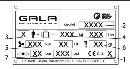
The indications on the capacity plate give information about limitations imposed by international regulations. Your local regulations can be different. Also these indications are not a complete list: the security requirements (obligatory security equipment of the boat, maximum authorized distance you can navigate from a shelter, etc.) may change according to the country or state.
